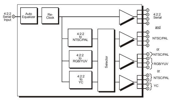
Figure 4-1. USM-6800 Functional Block Diagram
